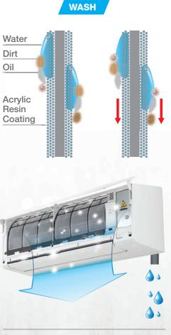
Reduces water and oil formation and prevents dust sticking to the coil units
