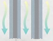
The fan operation after shut down helps dry water droplets to keep the coils dry and clean
